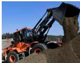
**Parallelkinematik (Tool Carrier)**
