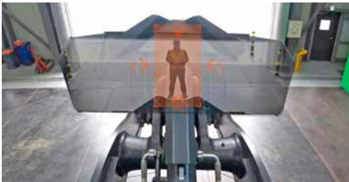
Another advantage of the transparent bucket system is that it can significantly improve work efficiency by providing a forward-view perspective for the driver during loading/unloading or when carrying materials such as aggregates, sand and soil.
