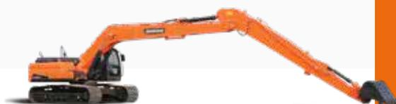
**Super-long reach and two-piece boom:** one long-reach machine – with a reach of 17.5 m – is ideally suited for special applications. A two-piece boom machine configuration is also available for more versatility.
