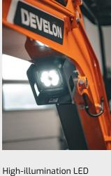
High-illumination LED lamps provide enhanced visibility to the work area to ensure that you can see the work group, particularly the attachment.
