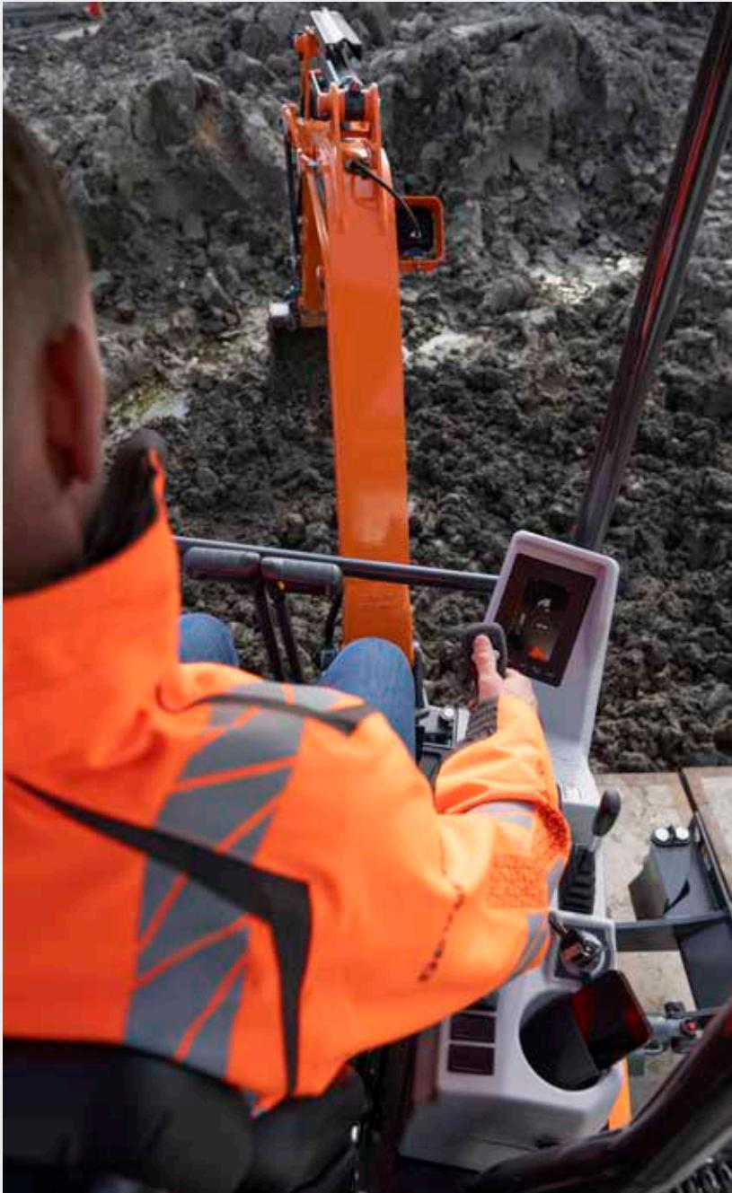
Highly sensitive, low-effort joysticks and clear convenient controls enable you to work safely, smoothly & confidently with minimum effort. Proportional auxiliary flow means precision control, smoothness & efficiency when using attachments.
