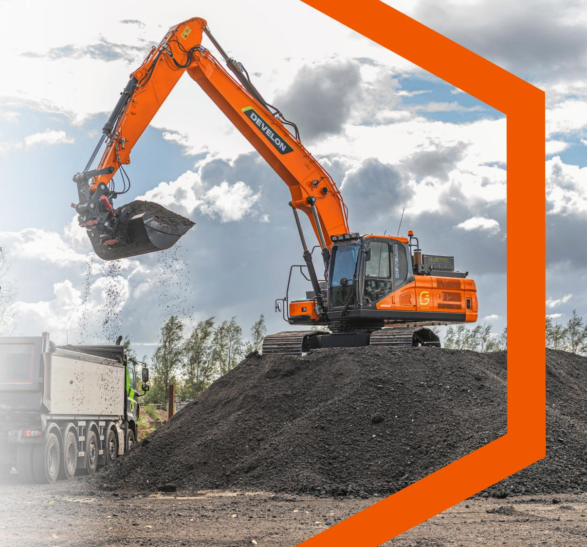
With a 120 kW liquid-cooled permanent-magnet motor, high-capacity LFP battery, and strong hydraulics, the DX230LCE-7 and DX250LCE-7 match comparable diesel crawler excavators — only quieter and emission-free at the point of use — so you can work where diesel is restricte keep noise low on urban sites, and still get the responsiveness, force, and attachment capability your business demands.
