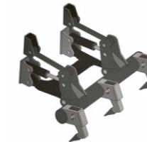
The Develon dozer comes equipped with piping for the easy integration of an optional parallel 3-shank ripper attachment. The ripper attachment features a parallel linkage that helps maintain a constant angle to the ground regardless of height. This attachment helps quickly break up hard, rugged materials before grading.
