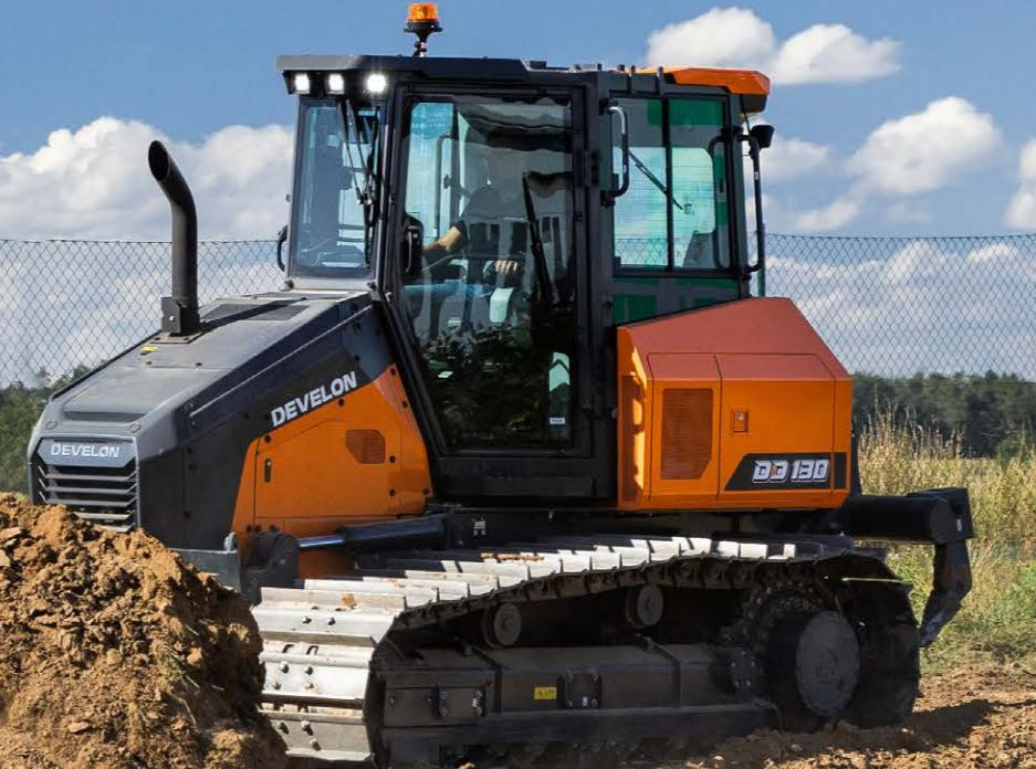
With a robust engine, a 6-way power tilt angle blade, and a lightweight build, our dozers aren't just strong—they're smart. Standard 2D Dozing Assist keeps your blade perfectly aligned for precise grading, and upgrading to 3D is seamless for even faster, more accurate work. They deliver power where and when you need it, while staying nimble enough for tight spots.
