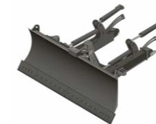
Choose from a standard (XL) blade or a low-ground pressure (LGP) configuration. See model spec sheets for blade capacity details.
