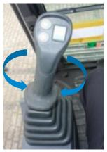
Joystick stroke angle reduced to 19° to reduce fatigue
