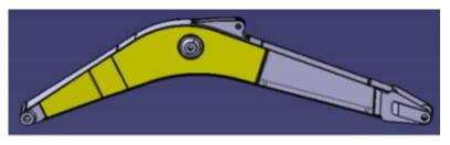
Boom: thickness of side plates increased by 20%
