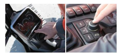
Easy navigation between functions directly on the instrument panel or via a joggle switch next to the joystick
